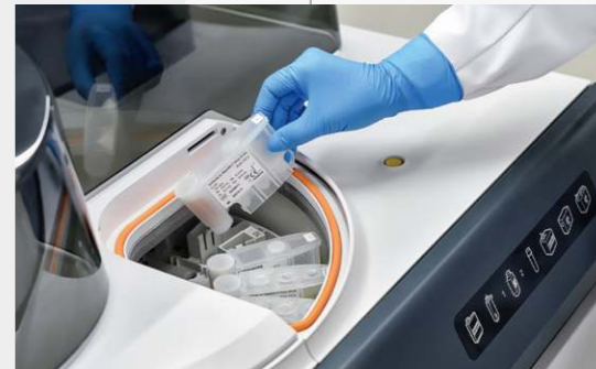
25 reagent positions with 2-8°C refrigeration
