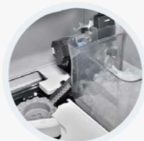
Bulk cuvette loader
